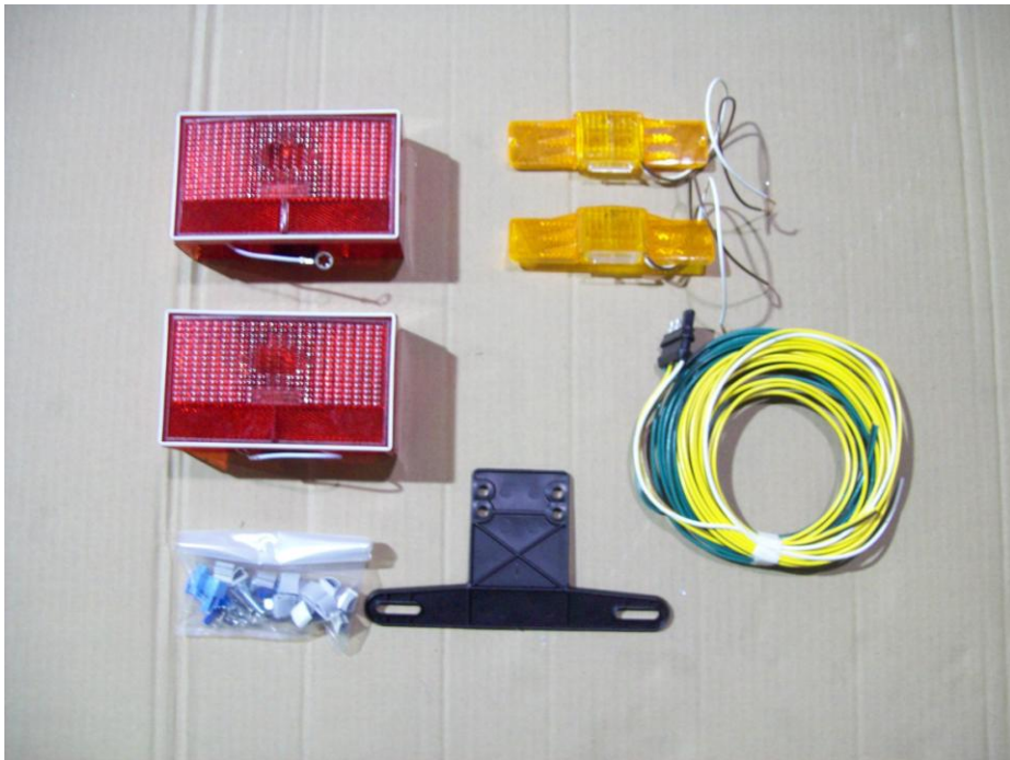
Tail lights, running lights, harness, license bracket and hardware
