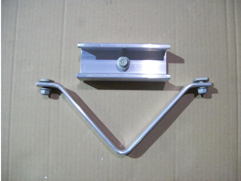
Skid and side marker light bracket
