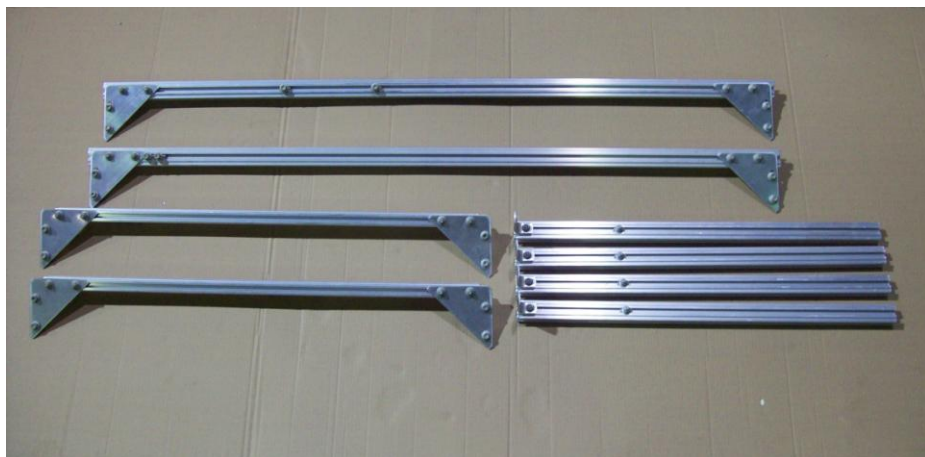
Top side rails, cross members and corner posts
